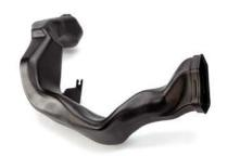
ROTATIONAL RIM (ROTO RIM) IS A UNIQUE PROCESS DEVELOPED AT RAPITYPES FOR THE MANUFACTURE OF HOLLOW COMPONENTS SUCH AS DUCTS, PIPES, AND AIR-BOXES. COMPONENTS CAN BE OF COMPLEX GEOMETRY WHILST ATTACHMENT BRACKETS AND FIXING DETAILS ARE FORMED AS PART OF THE COMPONENT.
